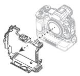
Then secure the cage by tightening the 1/4"-20 screw at the base with the Dual-Head Wrench.
